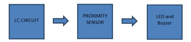
The LC circuit is nothing but inductor and capacitor which is connecter in parallel. The LC circuit will trigger the proximity sensor if it detects any metal near to it. Proximity sensor will give glow the led, and also make the buzz with the help of the buzzer.
